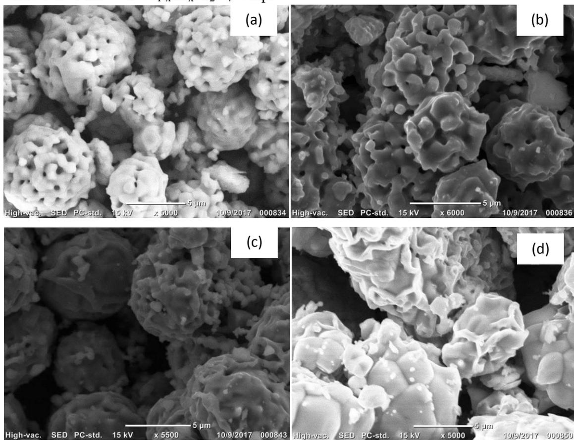
**Figure 3** SEM micrographs of  $\text{Co}_{1-x}\text{Zn}_x\text{Al}_2\text{O}_4$  where (a)  $x = 0.00$ , (b)  $x = 0.25$ , (c)  $x = 0.50$  and (d)  $x = 0.75$
