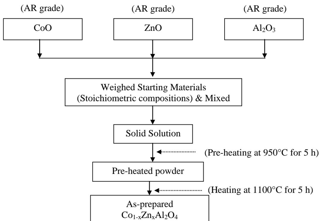
**Figure 1** Preparation procedure of  $\text{Co}_{1-x}\text{Zn}_x\text{Al}_2\text{O}_4$
