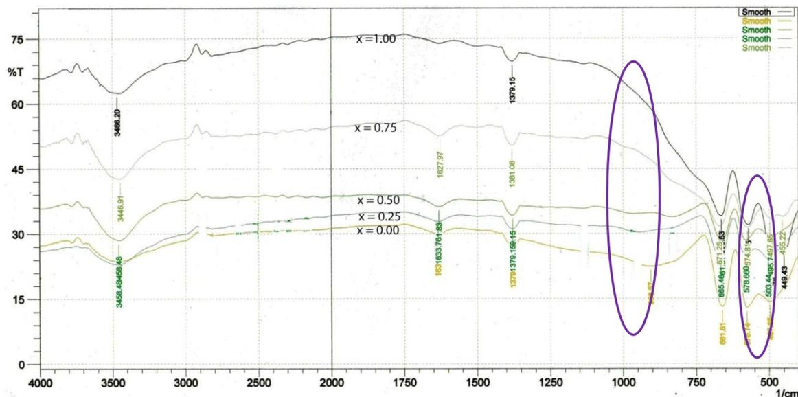
Figure 4 FTIR transmission spectra of  $Co_{1-x}Zn_xAl_2O_4$
