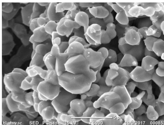
**Figure 3(e)** SEM micrograph of  $\text{Co}_{1-x}\text{Zn}_x\text{Al}_2\text{O}_4$  where  $x = 1.00$
