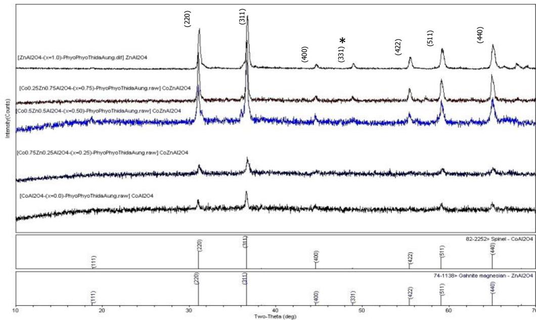
**Figure 2** XRD patterns of Co<sub>1-x</sub>Zn<sub>x</sub>Al<sub>2</sub>O<sub>4</sub>
